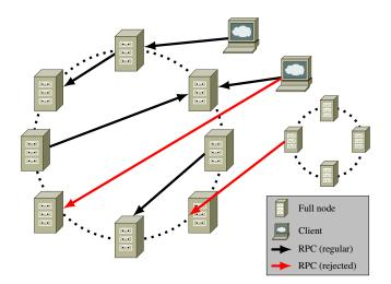
Fig. 4. Network architecture of *Fides*. The isolation prevents other full nodes within a different network of disturbing the ring structure. It is shown that full nodes are allowed to perform RPC calls when they are part of the network (inside the ring). Clients are only allowed to perform a subset of RPC calls on full nodes (outside the ring).
