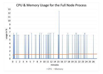
Fig. 5. CPU and Memory usage on a full node. The average memory usage is constant at about 1.1%, even with different transaction sizes during the measurement. The average CPU usage is 0.2%.
