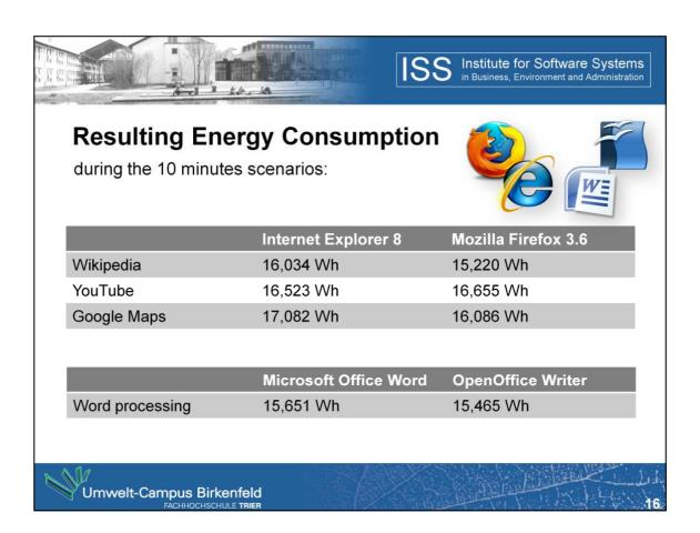
Overall, means over the testing period of 10 minutes the Internet Explorer consumed about 16 Watt hours.
