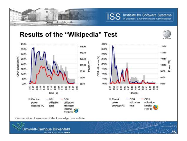
Comparing the results of testing the two internet browsers different values of energy consumption can be detected.
