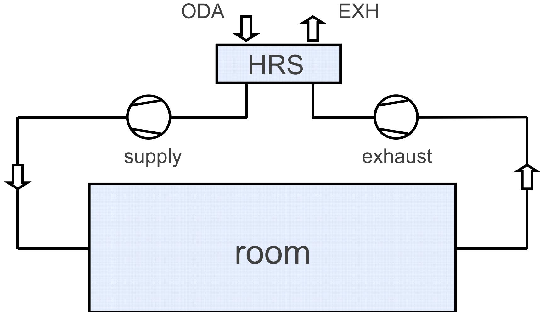
**Heat recovery** is the reusage of **thermal energy** by using the procedures of **heat transfer** in a process of minimum two mass flows with different temperatures.
