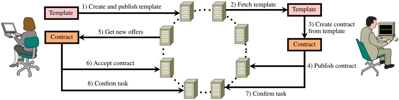
Fig. 7. General communication flow using the example of two clients. The person shown on the left creates a template, which is imported by the other person to create a contract from it. The processing takes place on the local objects, whose state is monitored by the distributed index. For simplicity, the arrows are used for transactions as well as for general requests to the network. The parties always use different full nodes to transmit their transaction to the network.
