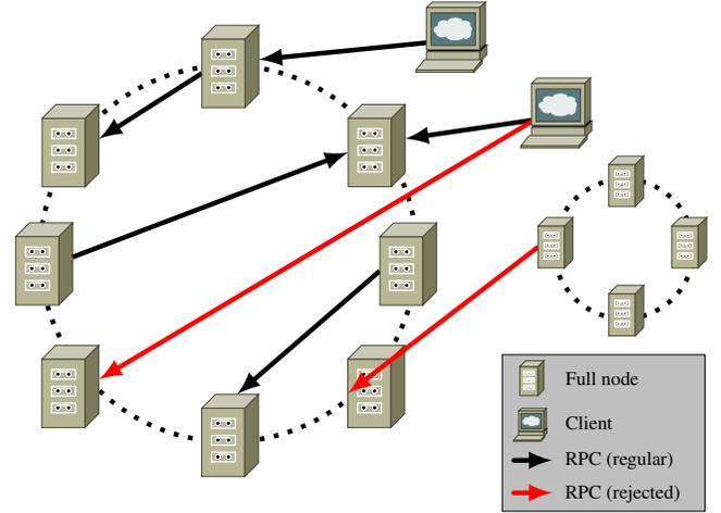
Fig. 4. Network architecture of *Fides*. The isolation prevents other full nodes within a different network of disturbing the ring structure. It is shown that full nodes are allowed to perform RPC calls when they are part of the network (inside the ring). Clients are only allowed to perform a subset of RPC calls on full nodes (outside the ring).
