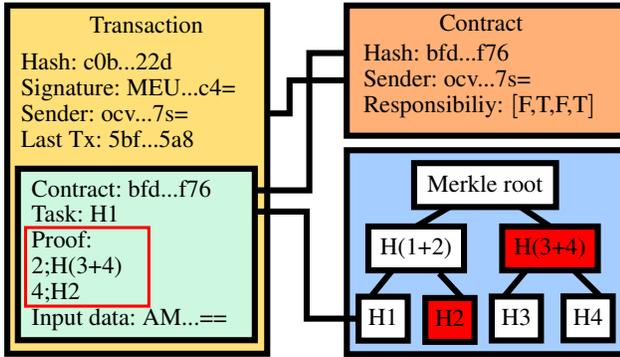
Fig. 2. An example of a simplified transaction that contains the necessary data to confirm a task in an active contract. The transaction addresses the previously created contract and the hash value of the task to be confirmed. Additionally included is the proof in the form of array elements and their position with respect to the full binary tree. Before any input is encrypted and added to the transaction, the validator assigned to that task will check the unencrypted input data.
