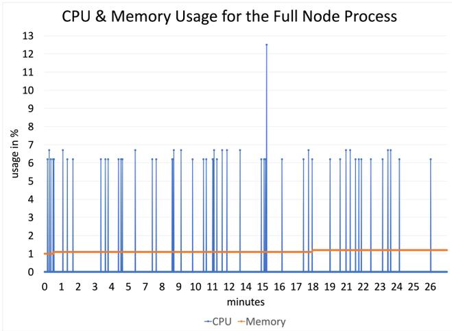
Fig. 5. CPU and Memory usage on a full node. The average memory usage is constant at about 1.1%, even with different transaction sizes during the measurement. The average CPU usage is 0.2%.
