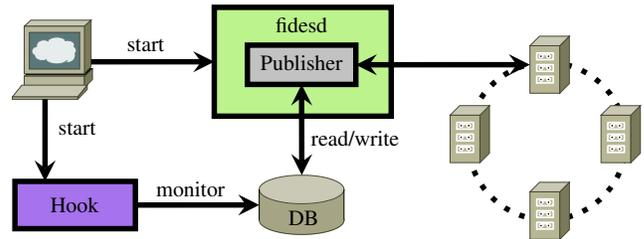
Fig. 8. Each Hook is independent of the core system and monitors the state of the database separately. The networking daemon is responsible for the communication with the network, whereby incoming or outgoing transactions change the state of the objects, causing the associated Hook to execute the contained callback.
